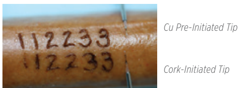
FIGURE 3. Comparison of cutting with a Cu pre-initiated tip (Top) and a cork-initiated tip (Bottom) at 1 W, 2 W, 3 W (Left to Right) CW
