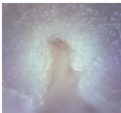
FIGURE 1. Cross-section of a cut made at 1.5 W, CW, 0.5 mm/s in pork muscle.
