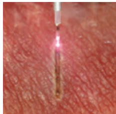
FIGURE 2. Still of Cu pre-initiated tip cutting beef tongue at 1.5 W, CW, 1.0 mm/s.
